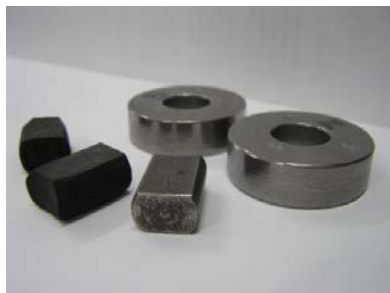
Fig. 12. Samples for measuring of wear resistance of details
