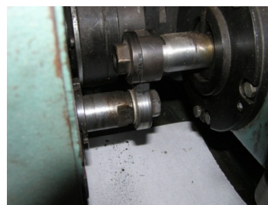
Fig. 4. Tests of materials on a wear at sliding and rolling friction with the pair of samples disk-rubber pad
